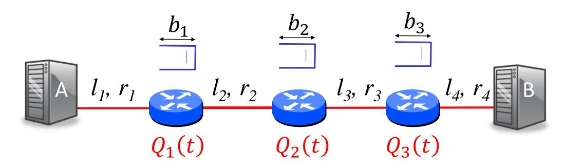
End-to-end delay for a single packet,  $\tau = \sum_{i=1}^{4} \left( \frac{p}{r_i} + \frac{l_i}{c} \right) + \sum_{i=1}^{3} Q_i(t)$  $\int \left(\frac{p}{r_i} + \frac{l_i}{c}\right) + \sum_{i=1}^{3} \frac{b_i}{r_i}$  $\leq \sum$
